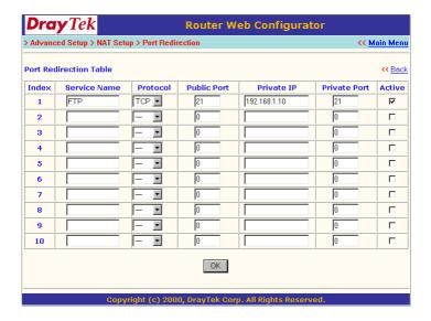
As shown above, the **Port Redirection Table** provides 10 port-mapping entries for internal hosts.
